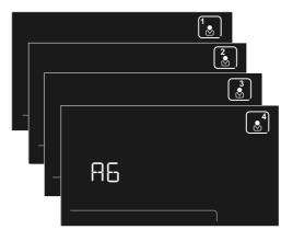
**Multi-profile feature.** Cuspidor-cup system automatisms, favourite working positions and settings for every single instrument can be saved for up to 4 different users, ensuring maximum versatility of use. This function is useful in multi-dentist surgeries or in clinics where there is high turnover of specialists.
