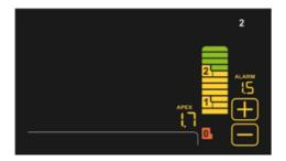
Apex locator. The apex distance is displayed on the LCD during the root canal instrumentation phase. The nearing of the apex is verified by the ENDO software. Once the apex is reached the Apex-Stop function interrupts micromotor rotation.
